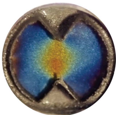
Figure (5) Over Tightened Indicator showing Yellow and Red
