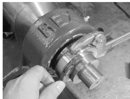
Figure (1) Wrench positioning to prevent sleeve from slipping
