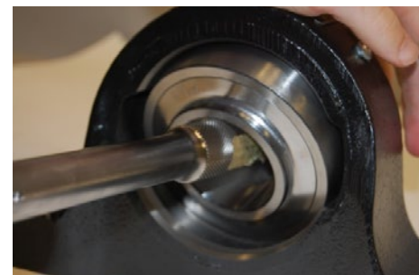
Figure 4 — Torquing bearing 90° into housing
