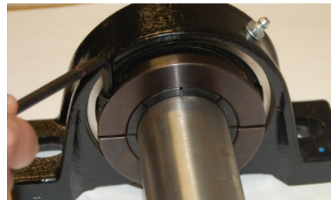
Figure 1 — Set screw tightening on a Centrik-Lok bearing
