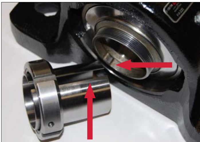
Figure 3 — If sleeve is removed from inner ring align spline with slot in sleeve to reinstall
