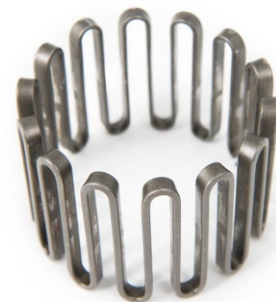
Falk grid element after 400,000 cycles
