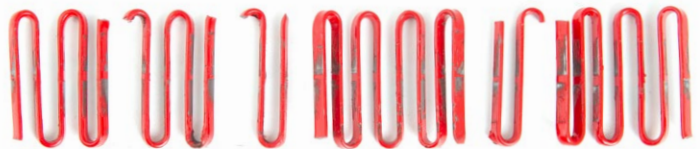
Dodge grid element after 70,000 cycles
