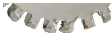
Continued use with broken grid elements will lead to complete destruction of hub teeth.
