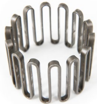
Falk® grid element after 400,000 cycles
