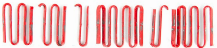
Dodge®* grid element after 70,000 cycles
