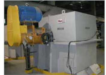
Shaft connection on a Rex® bucket elevator using a TLK132 internal locking device
