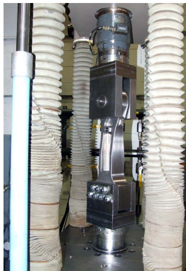
Fatigue Test of a Drag Brace
